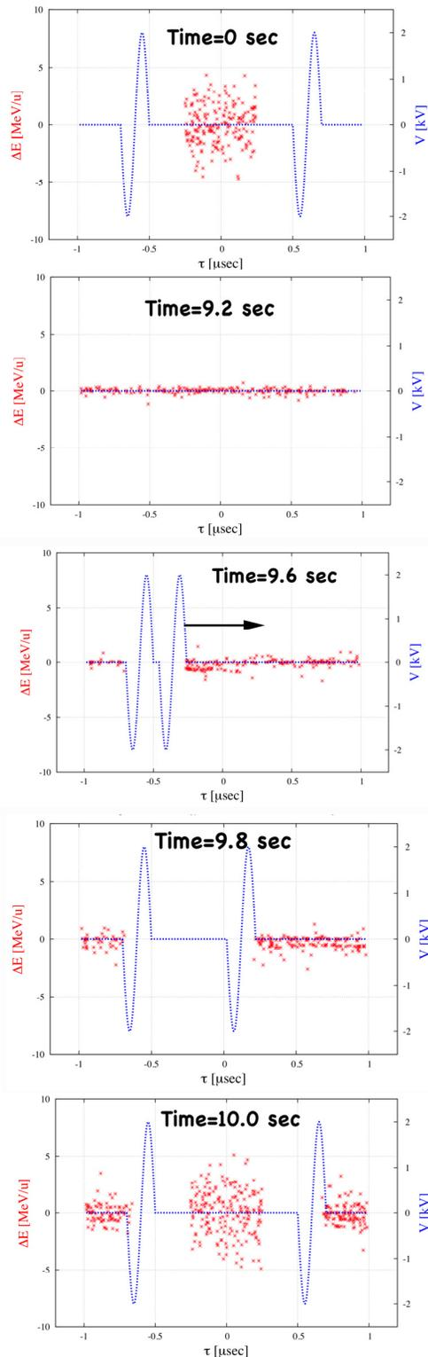
Figure 2: First cycle of antiproton accumulation with a moving barrier. At  $t = 9.5$  s the initially overlapping two barrier pulses are created. One barrier is then moved in the direction as indicated by the arrow. During the barrier motion the beam is compressed to provide new space for injection. The second batch is injected at  $t = 10$  s.
