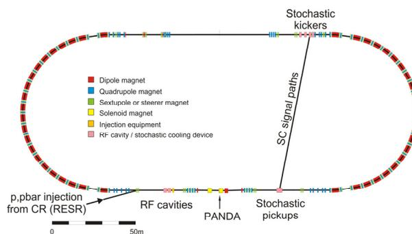
Figure 1: Schematic view of the HESR. The upper straight will accommodate the future electron cooler.
