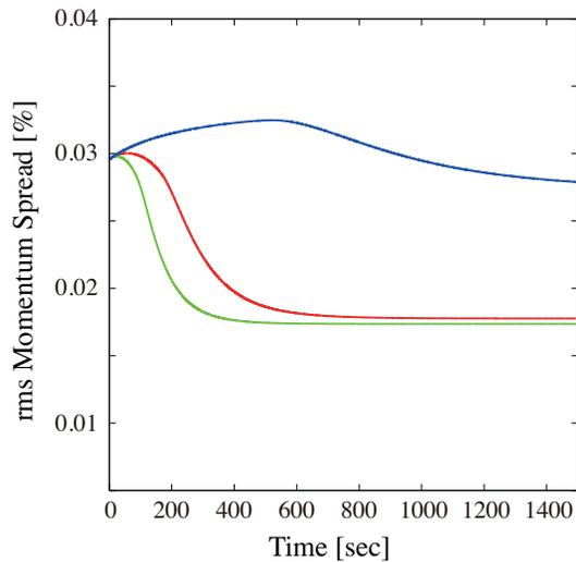
Figure 1: Momentum spread history with simultaneous use of stochastic and electron coolers. The red, green and blue curves show the results with the transverse stochastic cooling time of 250 sec and 100 sec, and without the transverse stochastic cooling ( $\tau_c = \infty$  sec), respectively.
