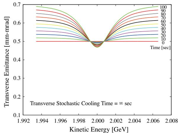
Figure 4: Transverse emittance during simultaneous use of stochastic and electron coolers for the transverse stochastic cooling time  $\tau_c = \infty$  sec (without transverse stochastic cooling).
