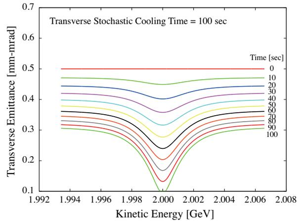
Figure 3: Transverse emittance during simultaneous use of stochastic and electron coolers for the transverse stochastic cooling time  $\tau_c = 100$  sec.
