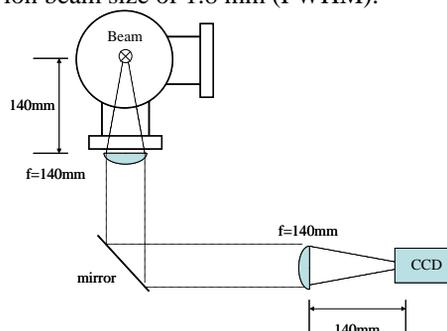
Figure 5 Observation scheme of the horizontal beam size of  $^{24}\text{Mg}^+$  ion beam.
