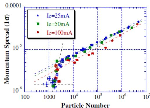
Figure 2 Demonstrated one dimensional ordering by electron beam cooling [2].
