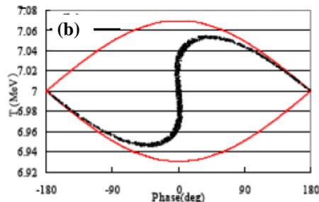
(b) Illustration of the phase rotation scheme after electron cooling to create a short bunch beam after electron beam cooling.
