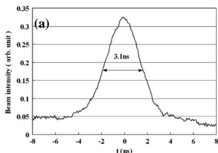
Figure 3(a) Realized shortest proton bunch (3.1 sec. at  $2\sigma$ ) by application of phase rotation as illustrated in (b).
