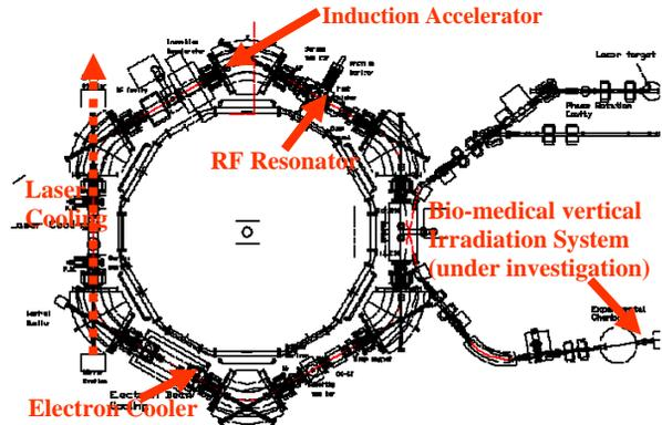
Figure 1: Electron Cooling and Laser Cooling system at S-LSR.
