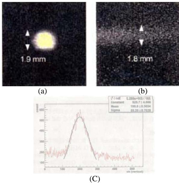
Figure 6 (a) Transverse laser profile (FWHM 1.9 mm) used to measure the spontaneous emission from excited  $^{24}\text{Mg}^+$  ions, (b) Observed spontaneous emitted photons and (c) Fitted results of the observed photon intensity resulting in a horizontal beam size of 1.8 mm (FWHM).
