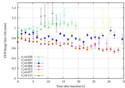
Figure 8 Time variation of the horizontal beam size for various synchrotron tunes.
