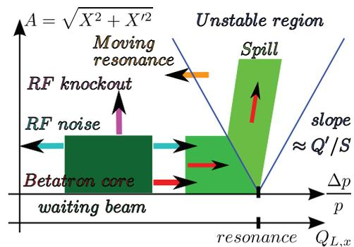
Figure 1: Steinbach diagram showing the various different driving mechanisms: a) betatron core (red), b) RF knockout (magenta), c) RF noise (cyan) and d) lattice tune adjustment (orange). The spill is indicated for case a and c.
