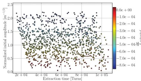
Figure 3: Correlation between initial normalized amplitude and extraction time for 400 MeV/u carbon ions with betatron core method, the extracted relative momentum deviation is color encoded
