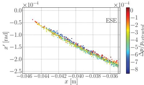
Figure 2: Phase space map ( $x-x'$ ) for betatron core method of extracted top energy carbon ions beam at ESE with the relative momentum deviation as color code. As expected, particles with high momentum exhibit the largest spiral step.
