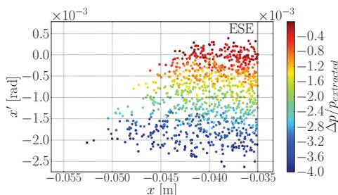
Figure 5: Phase space map ( $x-x'$ ) for lattice tune adjustment method of an extracted low energy proton beam at ESE with the relative momentum deviation color encoded
