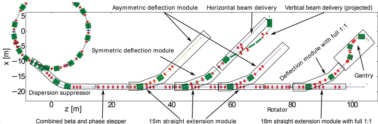
Figure 1: The layout of the MedAustron HEBT is built up from distinct functional building blocks.
