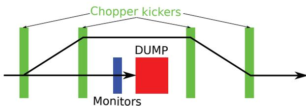
Figure 2: The 4 kicker beam chopping principle.
