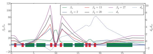
Figure 4: Beam optics of the vertical beam line as an example of a normal 1 : 1 module for various operationally-used vertical  $\beta_y$  functions. In the horizontal plane, the Twiss functions are constant as the beam size at the IR is adjusted by the rotation of the bar-of-charge in the horizontal phase space.
