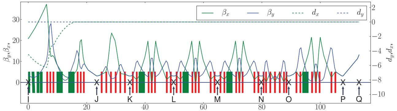
Figure 5: The optics of the main extraction line is built up from a dispersion suppressor (I - J), a beta and phase stepper (J - K) and a number of telescopic modules. The configuration of  $\beta_y = 3$  at the exit of the beta and phase stepper is shown.
