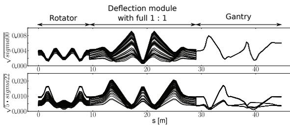
Figure 7: The beam size in the section from the rotator to the focal point for various gantry angles. (beam sizes are described by the  $\sigma$  matrix formalism)
