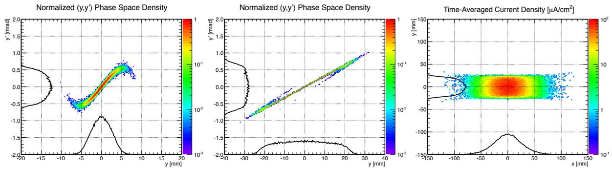
Figure 4: TraceWin [5] simulations based on transporting  $10^5$  particles. Left Panel: the  $(y, y')$  phase space distribution at the exit of the octupole,  $s = 0.8$  m. Middle panel: the  $(y, y')$  phase space distribution at target,  $s = 34.7$  m. Right panel: the  $(x, y)$  distribution on target has a Gaussian horizontal profile and an almost uniform vertical profile.
