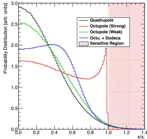
Figure 2: Normalized transverse distributions on the proton beam window/target for various expander systems. In all cases, the sensitive region is struck by less than 1% of the particles.
