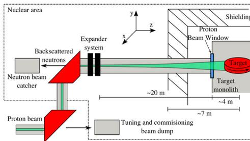
Figure 1: A sketch of the last part of the HEBT and target.
