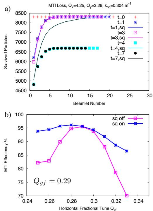
Figure 5: Skew quadrupole effect on a) beam loss and b) multi-turn injection efficiency.
