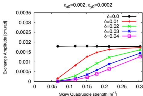
Figure 2: Emittance exchange amplitude versus skew quadrupole strength for different detuning.
