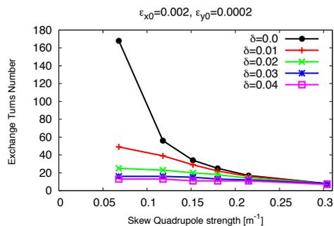
Figure 3: Emittance exchange turns number versus skew quadrupole strength for different detuning.
