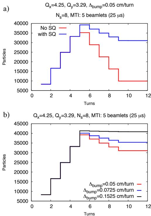
Figure 4: Bump speed optimization for one test working point with and without skew quadrupole.
