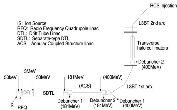
Figure 1: Schematic layout of J-PARC Linac upgrade, especially for debuncher system (dashed: ACS and new debuncher system for 400 MeV upgrade)
