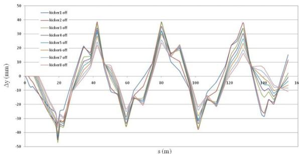
Figure 10: RTBT orbit due to extraction kickers misfire.
