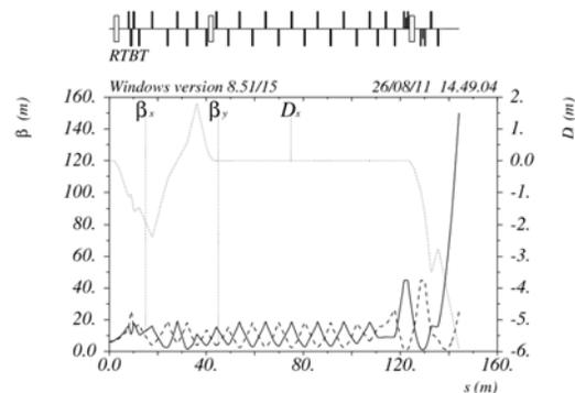
Figure 3: Linear lattice of RTBT.
