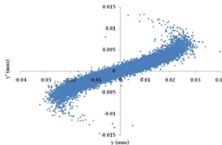
Figure 7: Particle distribution in vertical phase space at the target.
