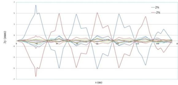
Figure 9: RTBT orbit variation due to extraction kickers wobble.
