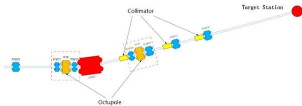
Figure 4: Arrangement of magnets for beam density redistribution.
