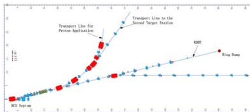
Figure 2: Layout of the transport lines to the second target station and proton application station.
