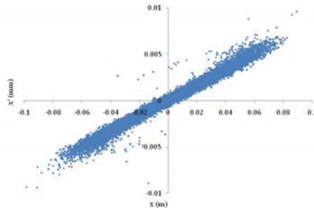
Figure 6: Particle distribution in horizontal phase space at the target.
