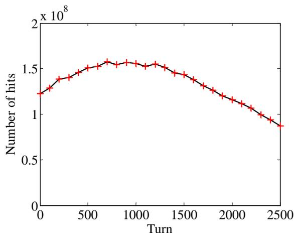
Figure 4: Number of hits on the foil at each turn during the extraction process.
