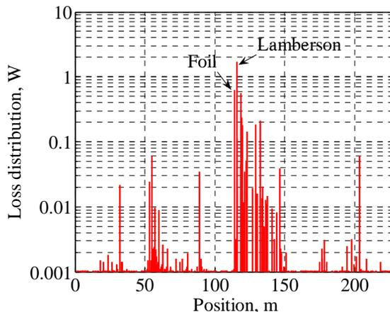
Figure 7: Beam loss distribution around the ring due to the foil scattering.
