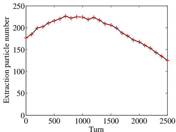
Figure 6: Number of extracted protons per turn.
