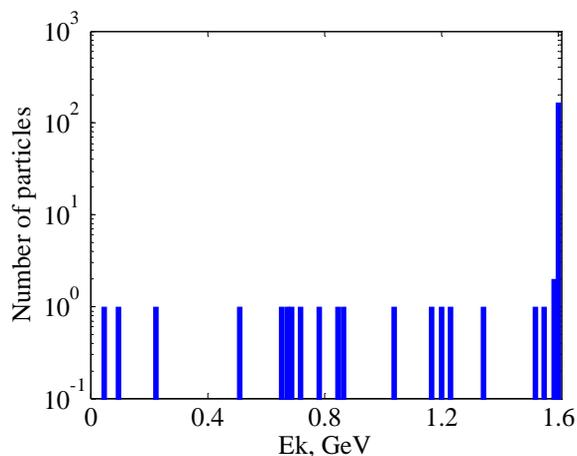
Figure 5: The energy distribution of the extracted particles.
