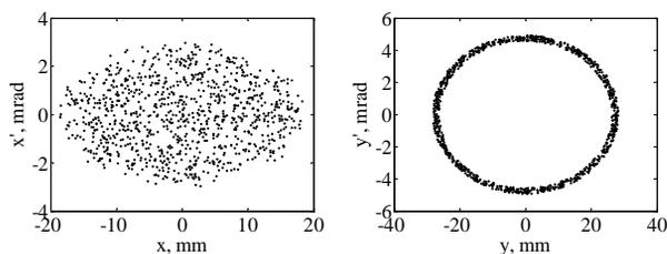
Figure 3: Distributions of the halo particles in the horizontal (left) and the vertical (right) phase spaces.
