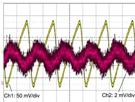
Figure 6: Voltage wave from the buncher (sawtooth in yellow colour) and the bunched-beam signal displayed on an analogue scope.
