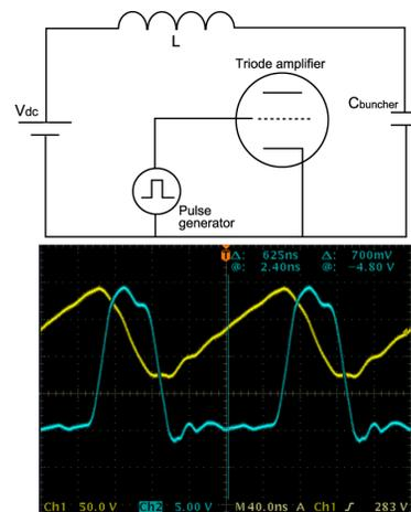
Figure 5: Top: Circuit diagram of the rf driving system for the rf buncher. Bottom: Voltage waves from the pulse generator (blue) and the buncher (yellow).
