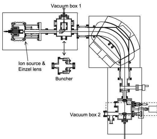
Figure 1: Configuration of the injection beam line.
