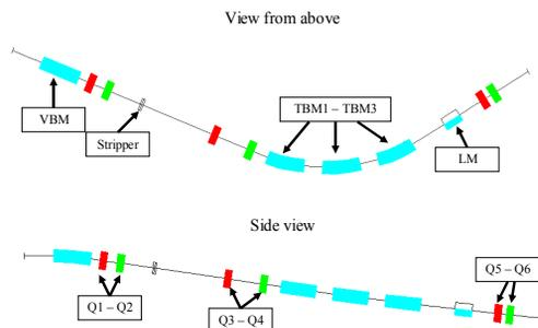
Figure 4: Scheme of Booster-Nuclotron beam line
