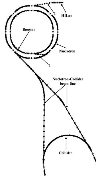
Figure 1: Scheme of NICA accelerator complex. 1 – HILac-Booster beam line, 2 – Booster-Nuclotron beam line.
