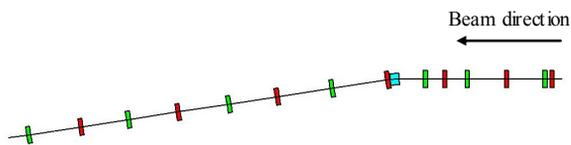
Figure 2: Scheme of HILac-Booster beam line. Red rectangles – focusing lenses, green ones – defocusing lenses, cyan one – bending magnet.
