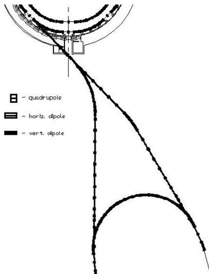
Figure 5: Scheme of Nuclotron-Collider beam line.
