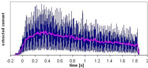
Figure 5: Extracted beam current, the pink line is the current averaged over 20 ms, i.e. without 50 Hz harmonics. All elements are static during extraction. The noise is caused by ripple on the supplies for the main quadrupoles and dipoles.
