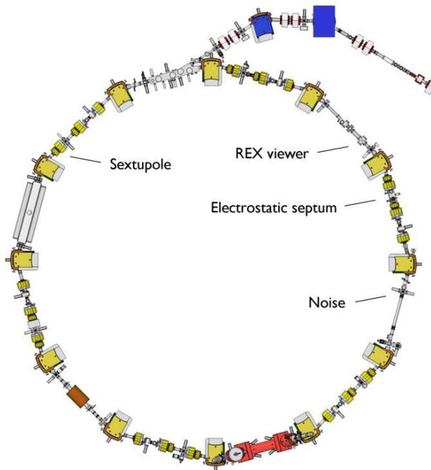
Figure 4: Hardware used for the tests of slow extraction.
