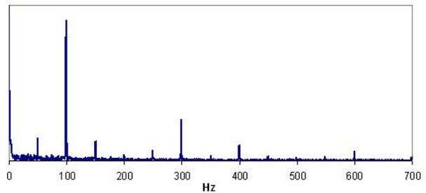
Figure 6: FFT of the beam current in the previous figure, 100 Hz and 300 Hz are the strongest components.
