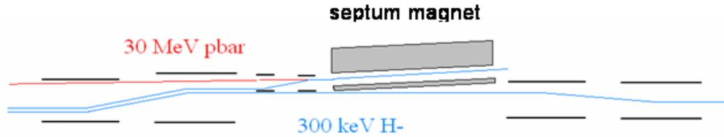
Figure 2: Bird's-eye view of the injection section. The path for single-turn injection of 30 MeV antiprotons is shown in red and the one for multiturn injection of 0.3 MeV protons in blue. The transverse scale is exaggerated for clarity. From left to right, two electrostatic kickers, two small electrostatic bends, septum magnet, two pairs of electrostatic kickers. Electrostatic elements are for slow ions only.
