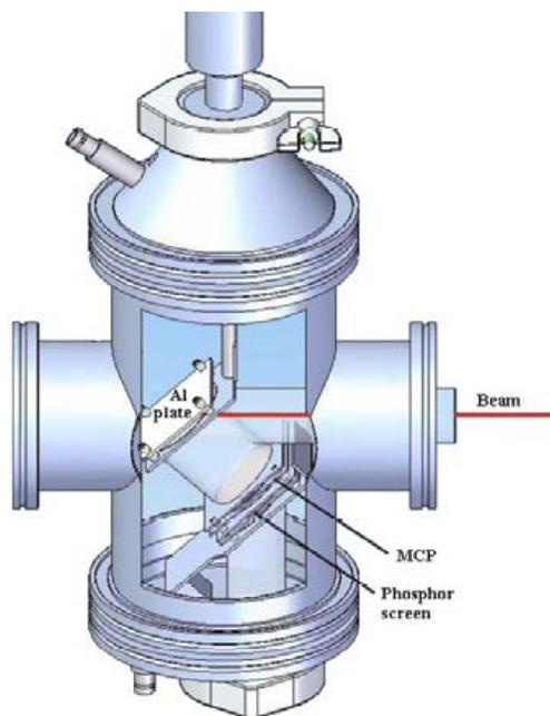
Figure 3: Drawing of REX-type beam viewer, where the beam comes in from the right, hits an aluminium plate and produces electrons that are amplified by MCPs and detected on a phosphor screen.
