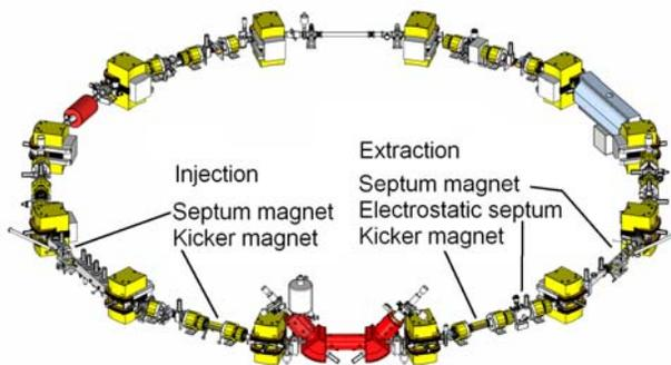
Figure 1: New hardware for injection and extraction.
