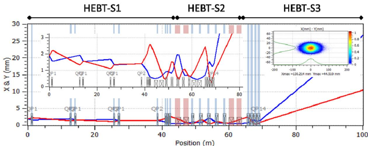
Figure 2: The horizontal (blue line) and vertical (red line) beam sizes (1rms) throughout the HEBT based on a multi-particle simulation of 100.000 particles. The colours denote the type of magnetic element: red = dipoles and blue = quadrupoles. The insets show a zoom-in of the beam sizes (left) and the particle distribution at the target (right).
