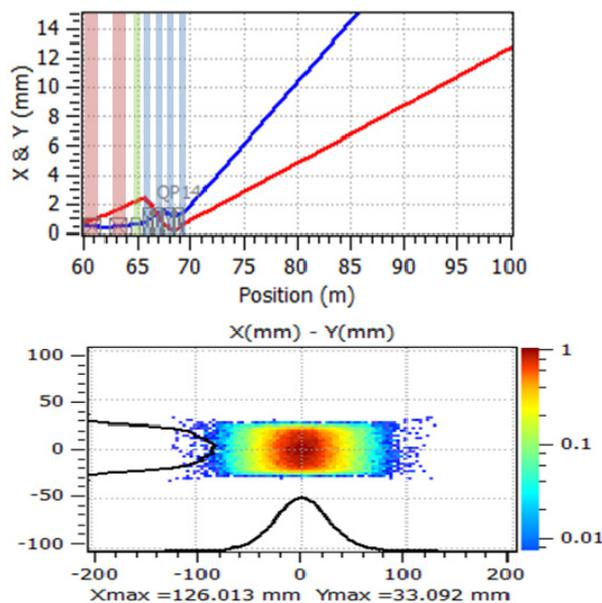
Figure 3: Top: The horizontal (blue line) and vertical (red line) beam envelopes from the position of the last two bending magnets of HEBT-S2 to target, the colors denote the type of magnetic element: red = dipole, blue = quadrupole, and green = octupole. Bottom panel: The beam intensity distribution at target.
