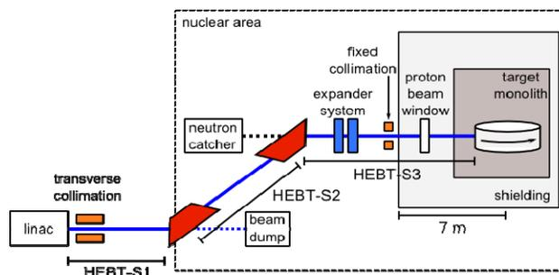
Figure 1: Layout of the linac to HEBT to target interface.
