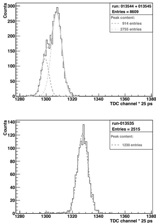
Figure 5: The *tof* spectra of ions for the carbon (*top*) and beryllium (*bottom*) peaks resulting from fragmentation of the primary Pb beam at 13.9A GeV/c. The spectrum of carbon is fitted by a sum of two Gauss functions, whereas that of beryllium by a single Gaussian.
