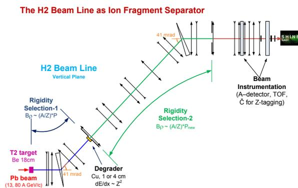
Figure 1: Schematic view of the vertical plane of the H2 beam line, relevant for the ion fragment separation.
