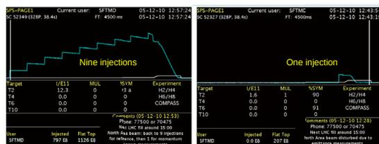
Figure 2: Screen shots of the SPS Page 1 illustrating an SPS cycle with nine (*left*) and one (*right*) injections of Pb ions at 13.9A GeV/c.
