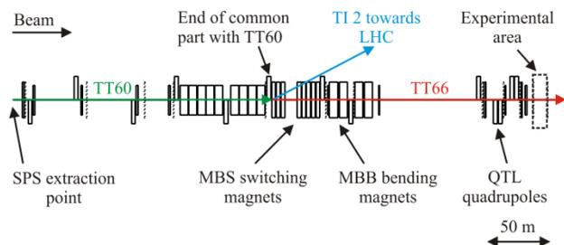
Figure 1: Layout of the HiRadMat primary beam line.
