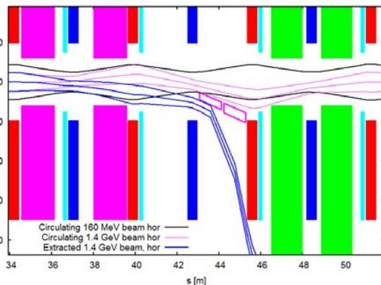
Figure 7: Extraction at 2 GeV kinetic energy from the RCS. The filled boxes in magenta and turquoise show the extraction kickers and bumpers and the magenta lines the septum blades. Beam envelopes (blue for injection energy, black for lowest extraction energy) are shown for a 3 sigma beam size including a closed orbit distortion of 1 mm.
