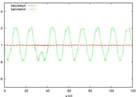
Figure 6: Beta beating for SBEND chicane and painting magnets.
