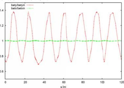
Figure 5: Beta beating for RBEND chicane and painting magnets.
