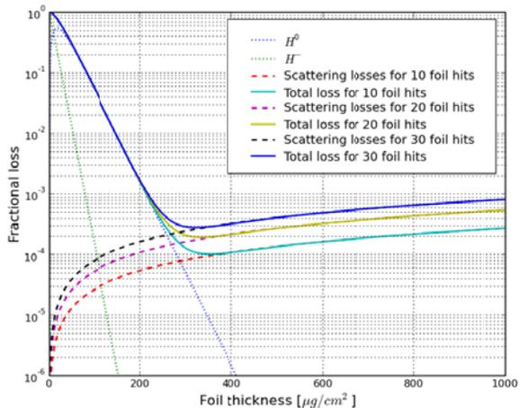
Figure 2: Optimisation of foil thickness with respect to beam losses from stripping efficiency and scattering. The optimum foil thickness is 350  $\mu\text{g}/\text{cm}^2$  for 10 foil hits per proton and 320  $\mu\text{g}/\text{cm}^2$  for 30 foil hits.
