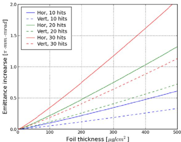
Figure 3: Emittance increase due to multiple coulomb scattering in the foil.
