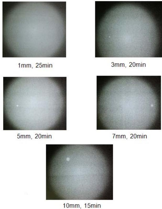
Figure 8: Artificial defects measured by 950KeV Linac with Imaging Plate.
