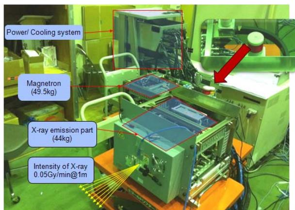
Figure 1: Upgraded X-band 950KeV Linac.
