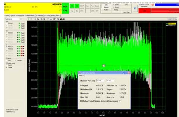
Figure 3: Spill shape for carbon beam with (green) and without (grey) feed back.
