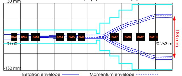
Figure 4: Beam envelope functions with kicks of the scanning magnets, located between BM6 and BM7.
