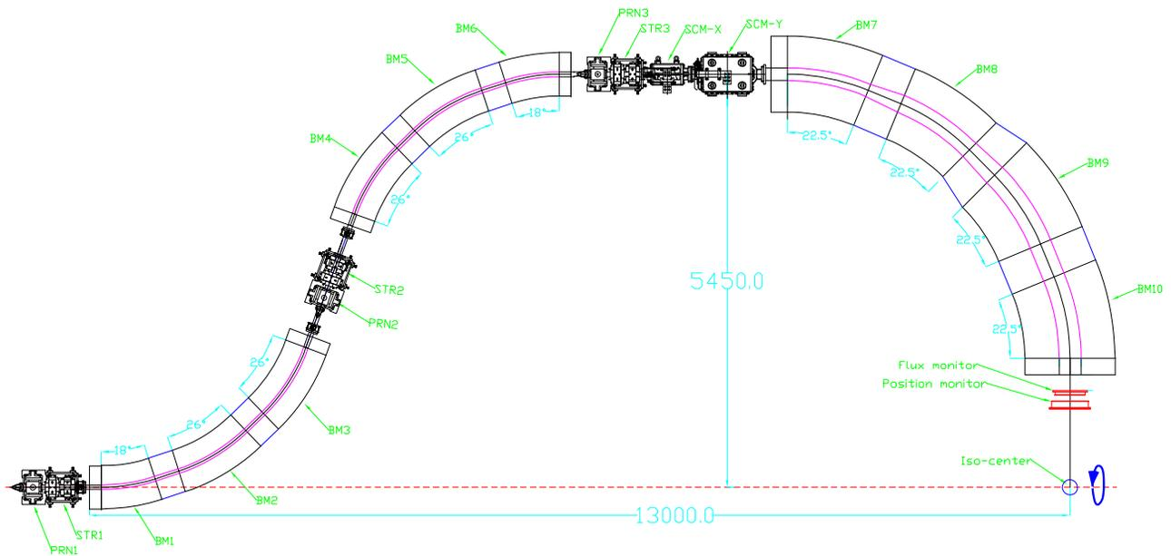
Figure 2: Schematic drawing of the rotating gantry for the heavy-ion therapy.
