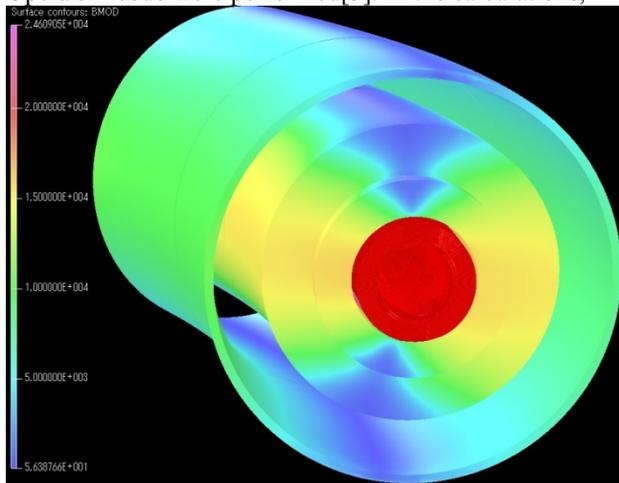
Figure 6: Result of 3D electromagnetic field calculation using the Opera3D code. A unit of the color map in Gauss.
