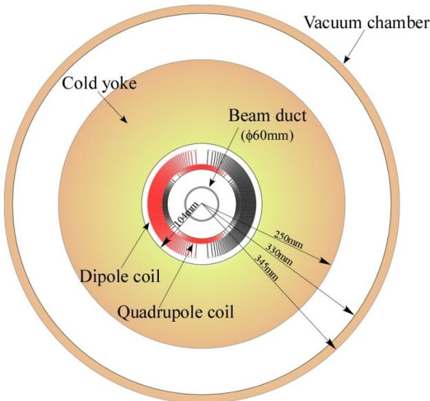
Figure 5: Cross sectional view of the superconducting magnet for BM1 through BM6.
