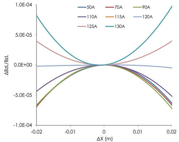
Figure 7: Uniformity of dipole field,  $\Delta B_z L/B_z L$ , for the various coil currents. The calculated  $B_z L$  was 3.03 Tm with the coil current of 130 A.,
