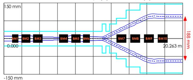
Vertical beam envelope [m] versus distance [m]
