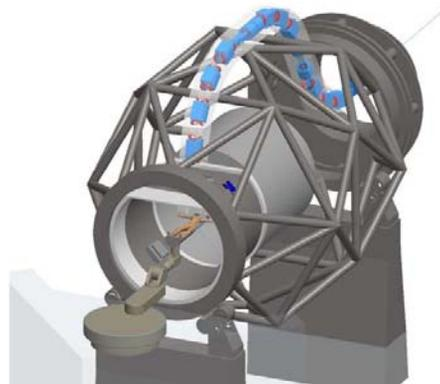
Figure 7: Schematic view of the superconducting rotation gantry for carbon beam.
