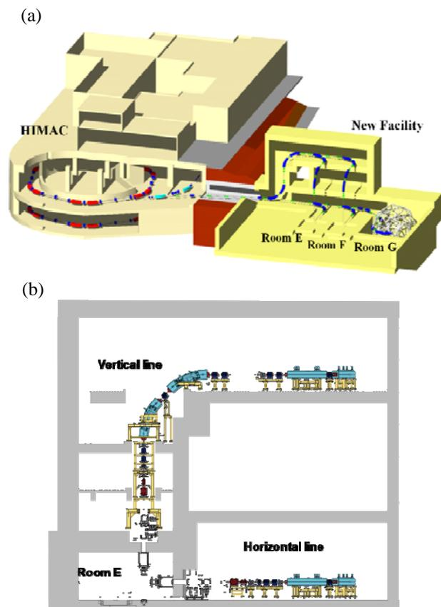
Figure 1: Schematic view of the HIMAC and New Particle Therapy Research Facilities (a), and the horizontal and vertical irradiation lines for the treatment room E (b).
