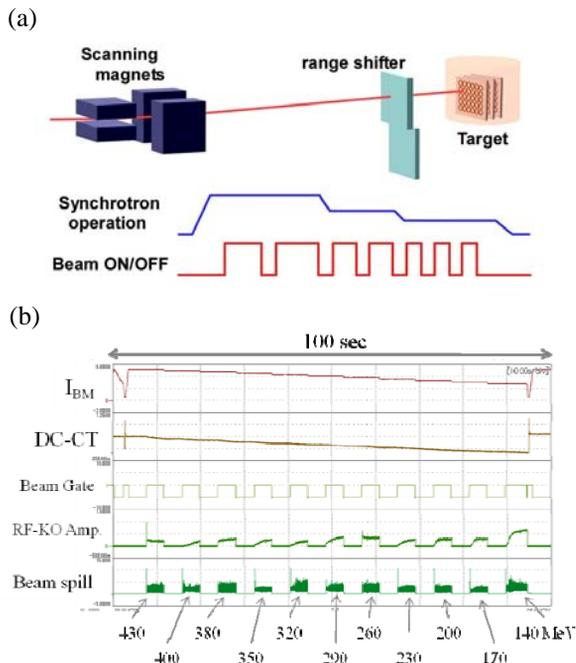
Figure 6: Scheme of the combination scanning (a) and the demonstration of the continuous change of the extracted beam energy (b).
