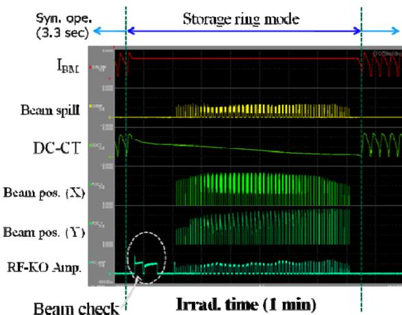
Figure 4: Typical operation pattern of the 3D scanning system.  $I_{BM}$  is the current of the bending magnets in the synchrotron. Beam positions are the measured values by the beam position monitors near the isocenter.
