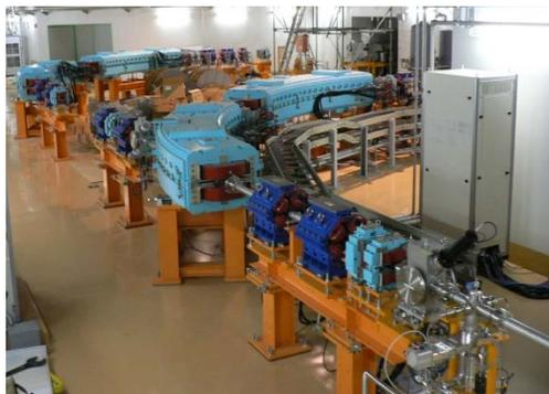
Figure 2: High energy beam transport line (horizontal).
