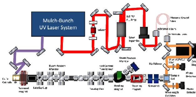
Figure 2: Experimental setup of pump-probe pulse radiolysis with SC
