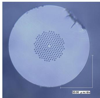
Figure 1: The cross sectional micrograph of PCF
