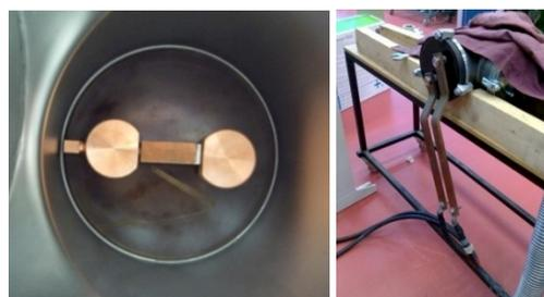
Figure 5: Inconel® RF-contact test bench.
