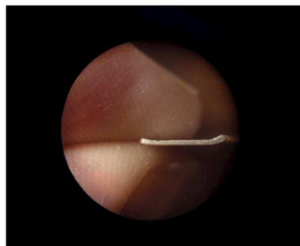
Figure 4: Cross section of Inconel® RF-contact.
