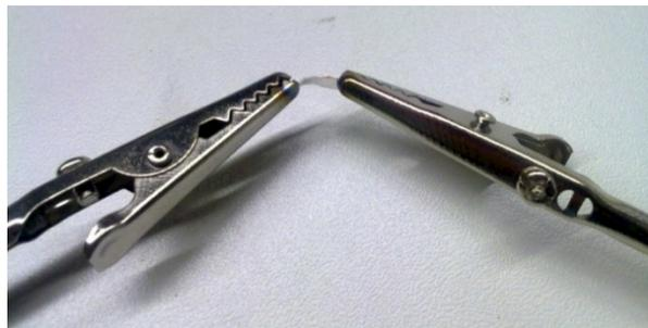
Figure 3: DC test of RF finger contact.
