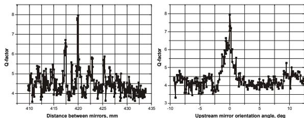
Figure 4: Cavity length and upstream mirror orientation angle scans.
