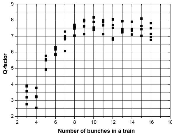
Figure 5: Dependences of the resonator Q-factor versus number of bunches in a train.
