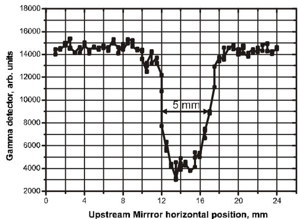
Figure 2: Dependences of bremsstrahlung measured by gamma detector versus horizontal mirror position.
