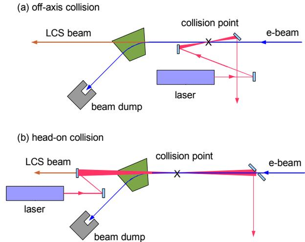
Figure 3: A schematic view of collision geometry. (a) off-axis collision and (b) head-on collision.
