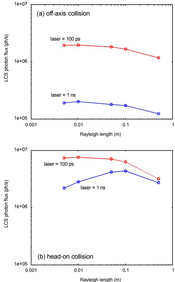
Figure 4: Calculated LCS photon flux for (a) off-axis collision and (b) head-on collision. The flux is integrated over the entire energies.
