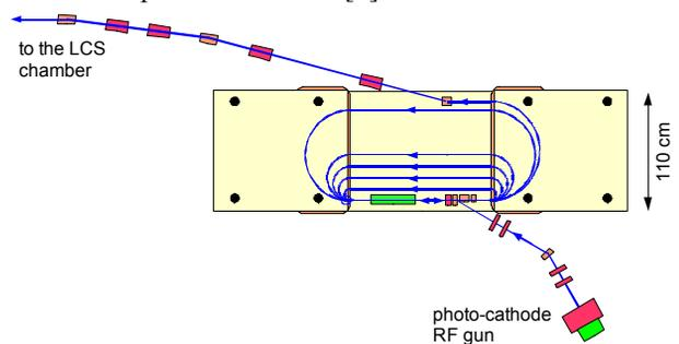
Figure 1: A schematic view of the 150-MeV racetrack microtron at JAEA Kansai.
