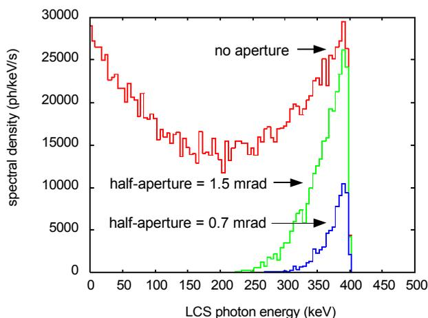
Figure 5: Calculated spectrum of LCS photons for the head-on collision with a laser pulse of 100 ps and Rayleigh length of 0.01 m.
