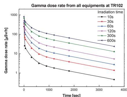
Figure 6: Gamma dose rate of all equipments at TR102.
