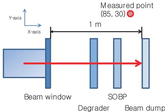
Figure 1: The schematic diagram for code simulation.
