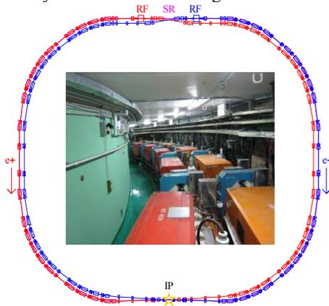
Figure 1: BEPCII layout and its real tunnel (blue: e<sup>-</sup> ring, red: e<sup>+</sup> ring)
