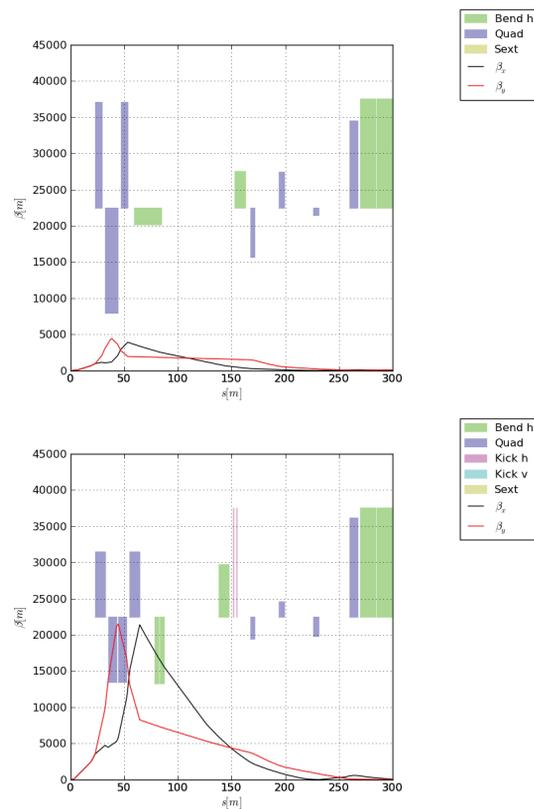
Figure 1: Nominal (top) and upgrade (bottom) IR1-5 layout and optics ( $\beta^* = 55$  cm and 15 cm, respectively).
