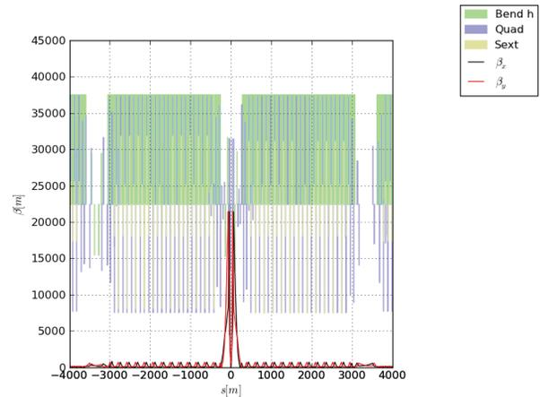
Figure 3: Nominal (top) and upgraded (bottom) collision optics for the low- $\beta$  IR and surrounding sectors.
