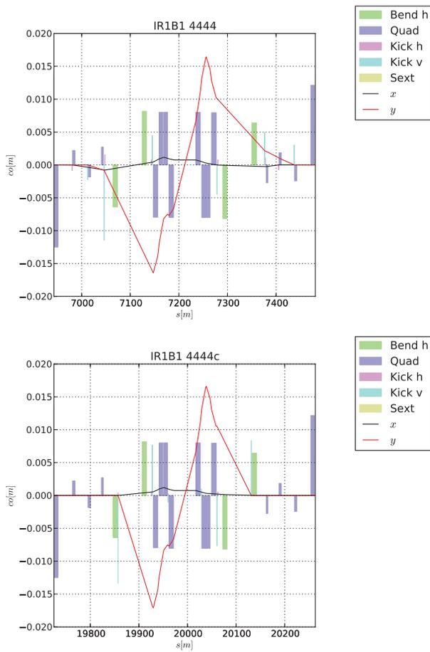
Figure 4: Baseline (top) and alternative (bottom) crossing parallel separation bumps, with corresponding orbit corrector strengths, for Beam 1 in IR1.
