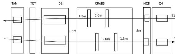
Figure 2: Tentative layout of the crab cavity area. The cavities of both beams are interleaved to equalize the voltage needed for Beam 1 and Beam 2 on the left and right sides of the IP. The assembly is pushed towards D2, and D2 is eventually pushed towards the IP to gain in voltage efficiency, thanks to larger beta functions.
