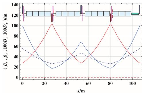
Figure 5: e-ring arc cell optics. One arc period consists of two asymmetric FODO cells. The horiz./vert.  $\beta$ -functions are shown in blue/red and the dispersion in dashed blue/red.
