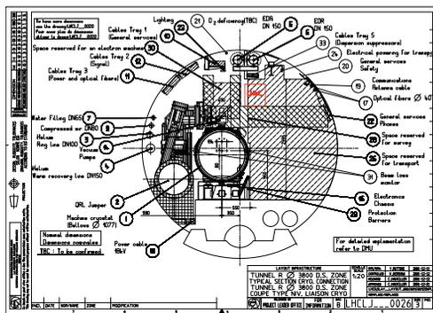
Figure 1: Cross-section of the LHC tunnel with the original space holder for the e-ring directly above the LHC cryostat and the shifted location (red) required to keep the overall circumference of e- and p-ring identical.
