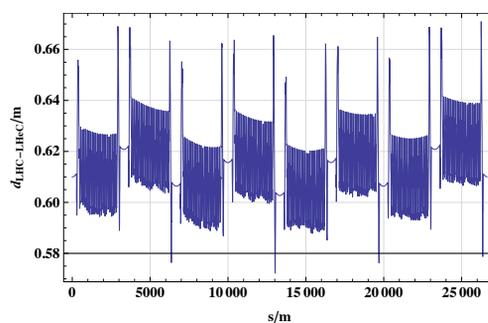
Figure 4: Radial distance between the p- and e-ring without bypasses.
