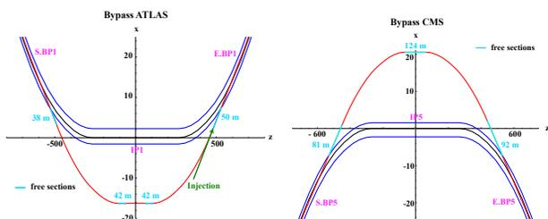
Figure 3: Final bypass design: The LHC p-ring is shown in black, the e-ring in red and the tunnel walls in blue. Dispersion free sections reserved for the installation of RF, wiggler(s), injection and other equipment are marked in light blue. The injection is marked in green in the right arc of the bypass in Point 1. Beginning and end of the bypass are marked as S.BP and E.BP.
