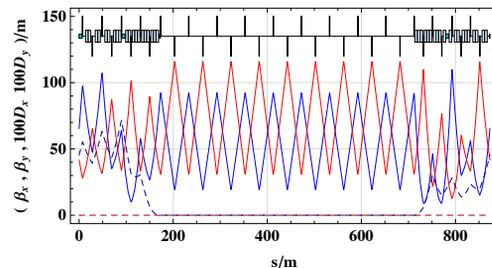
Figure 6: Insertion layout and optics at even points.
