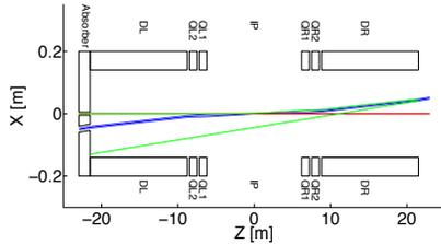
Figure 4: Radiation envelope for the high acceptance layout.
