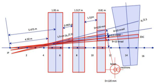
Fig. 3. Proton/ion eRHIC IR magnets.
