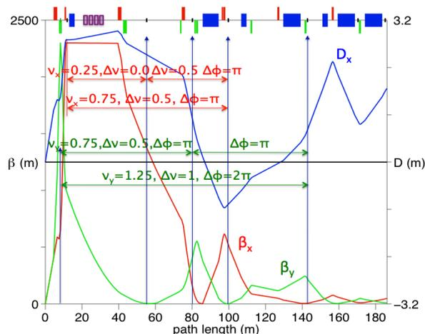
Fig. 11. Betatron functions in the half of the IR. The sextupole positions and their phase differences are marked with arrows.
