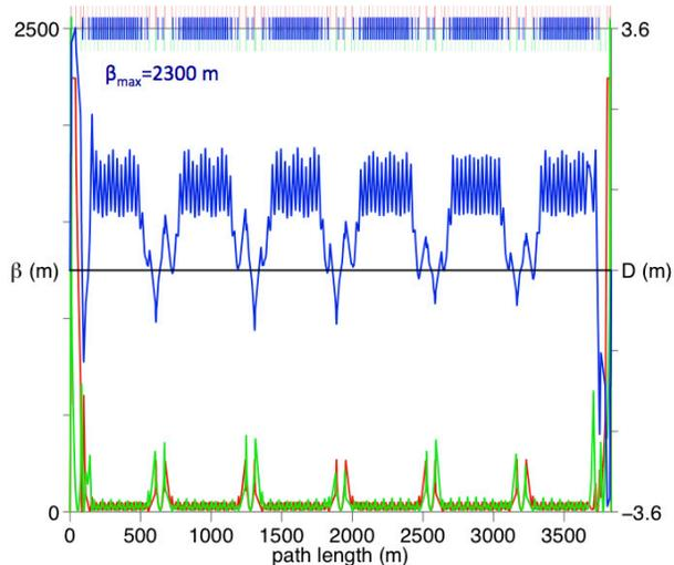
Fig. 8. The eRHIC lattice functions: the  $\beta_x$  is the horizontal; the  $\beta_y$  is the vertical betatron function, while  $D_x$  is the dispersion function.
