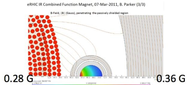
Fig. 6. Electron double shielded pipe in the combined function magnet. Electrons pass at 4.5 cm away from the axis.
