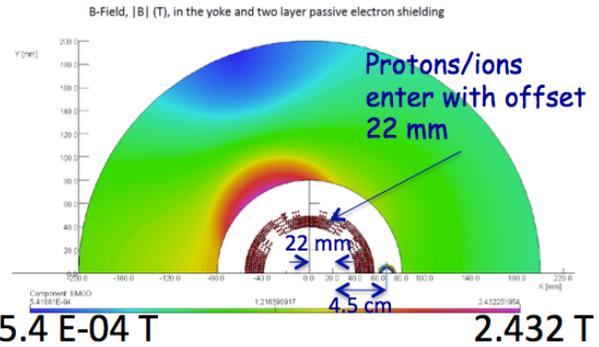
Fig. 5. A cross section of the combined function magnet. Protons/ions enter with 22 mm offset and are bent for 4 mrad.
