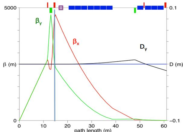
Fig. 9. Electron IR lattice functions.
