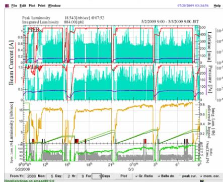
Figure 5: The luminosity changed on May 2nd 2009 when skew sextupole magnets were firstly used.
