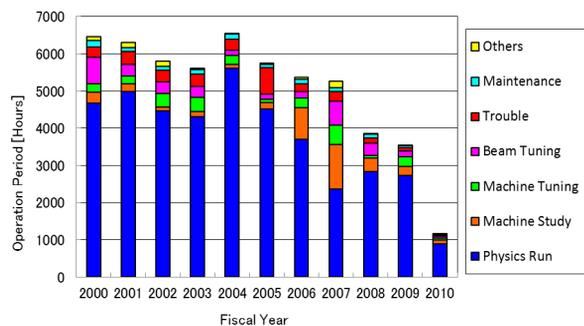
Figure 7: The use of available time for KEKB in hours.
