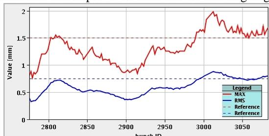
Figure 9: IQC plot of injection oscillation amplitudes and RMS for 144 bunches of a beam 2 injection. The difference between minimum and maximum amplitude is more than 1 mm.
