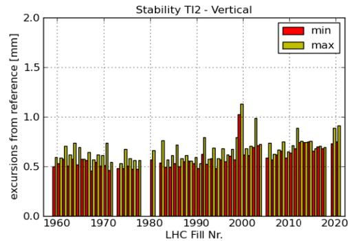
Figure 6: TI 2 Vertical: Minimum and maximum excursion from reference during fill.
