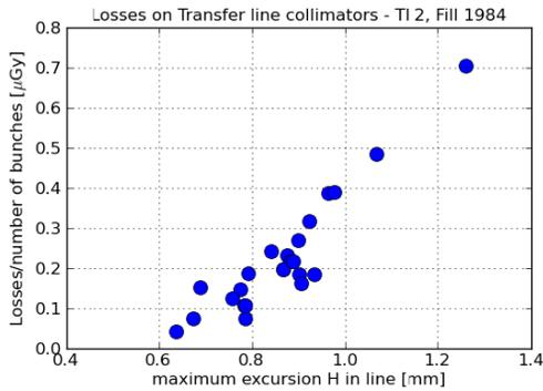
Figure 2: Correlation between maximum excursion in TI 2, horizontal, and total losses on transfer line collimators normalised to number of bunches.
