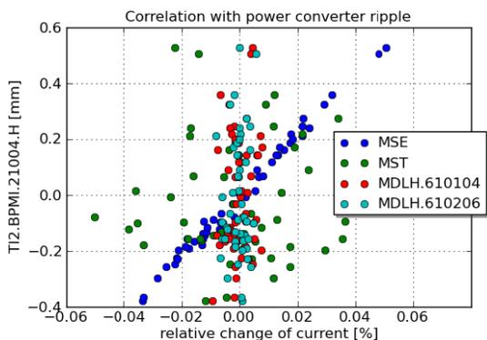
Figure 7: Simulation with MAD-X: excursion at TI 2 BPM versus measured power converter ripples of several dipole circuits at the beginning of TI 2. The MSE ripple correlates well with the BPM excursion.
