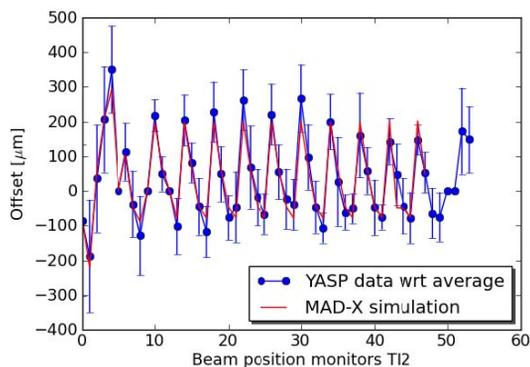
Figure 8: Measured trajectory in TI 2 with respect to average of extraction test period on 19<sup>th</sup> of June, 2011 and MAD-X simulation of expected trajectory with current error of MSE at the moment of the measurement.
