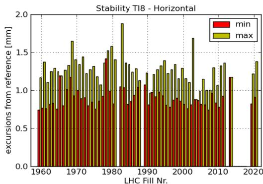
Figure 3: TI 8 Horizontal: Minimum and maximum excursion from reference during fill.
