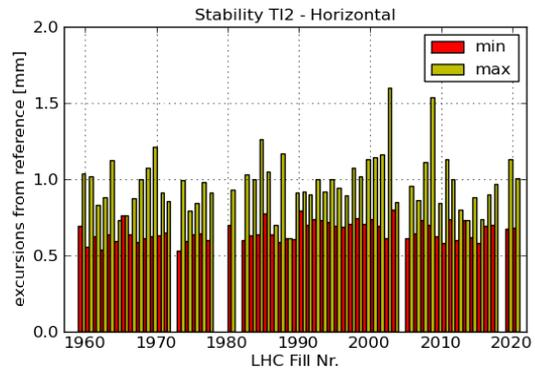
Figure 5: TI 2 Horizontal: Minimum and maximum excursion from reference during fill.
