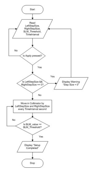
Figure 3: Semi- Automatic Algorithm Flowchart.
