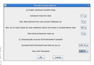
Figure 4: Parallel Collimator Setup Settings.
