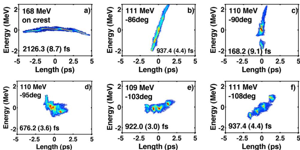
Figure 5: Four comb pulse longitudinal phase space rotation; the label reports the average energy, the compression phase and the rms bunch length (200pC).
