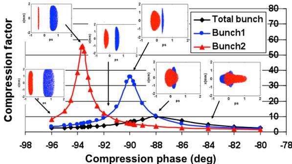
Figure 1: Compression curve for two bunches pulse train at SPARC (simulation, total charge 165pC).
