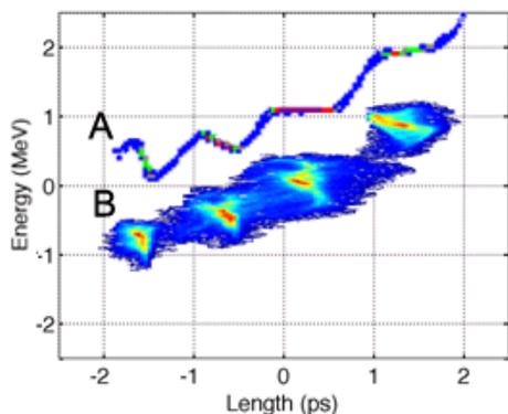
Figure 6: Comparison of measured longitudinal phase space (B) to simulated one (A). (200 pC)
