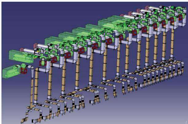
Figure 5: 3-D layout of the Linac4 RF system.
