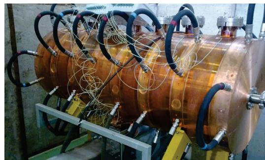
Figure 4: PIMS first cavity under high-power tests.
