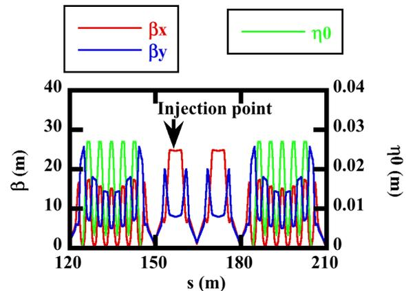
Figure 1: Lattice function of SPring-8 II.
