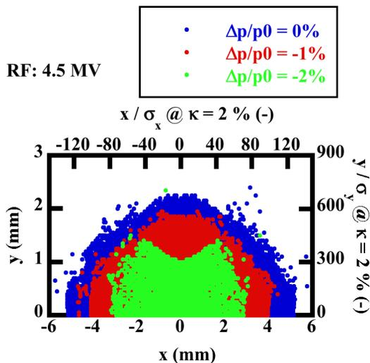
Figure 2: Dynamic aperture without error at injection point.
