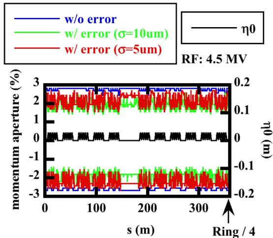
Figure 5: Momentum aperture with Sx-alignment error.
