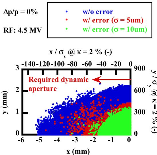
Figure 4: Dynamic aperture for on-momentum particles with Sx-alignment error at injection point.
