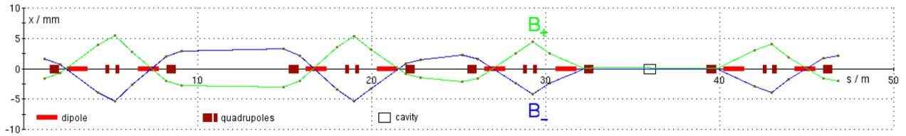
Figure 2: Measured dispersive orbit of the  $B_{\pm}$  electron beams with  $\alpha_1 = 0$ ,  $x$  describes the horizontal displacement,  $s$  the longitudinal position. The dispersion in the straight of the cavity (at  $s = 36$  m) is zero.
