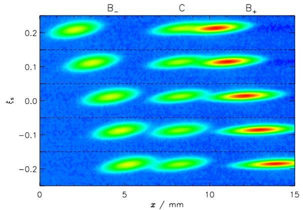
Figure 3: Triple beam measured by a source point imaging system at a  $D > 0$  location, while varying  $\xi_s$ .
