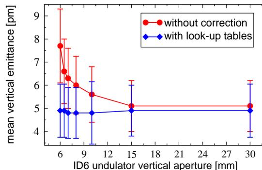
Figure 2: Mean vertical emittance  $\bar{\epsilon}_y$  measured against the vertical aperture of the ID6 in-vacuum undulator without any correction (red circles) and with automatic coupling compensation (blue diamonds). Error bars corresponds to the spread  $\delta\epsilon_y$ .
