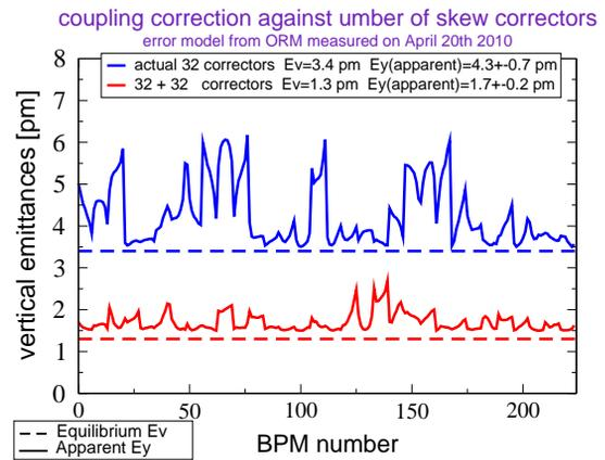
Figure 4: Simulation of vertical apparent and equilibrium emittance with the present coupling correction setting of 32 and its further reduction with 32 additional correctors.
