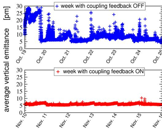
Figure 3: Comparison between the mean vertical apparent emittance  $\bar{\epsilon}_y$  measured towards the end of 2010 during beam delivery without (top) and with (bottom) coupling feedback. Data acquired during refills are not displayed.
