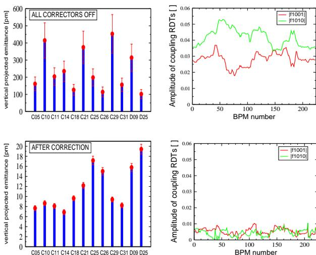
Figure 1: Vertical apparent emittances  $\mathbb{E}_y$  measured on January 16 2010 along the ESRF storage ring (ten dipole radiation projection monitors and two pinhole cameras) and corresponding coupling RDTs with all correctors off (top) and after correction (bottom).
