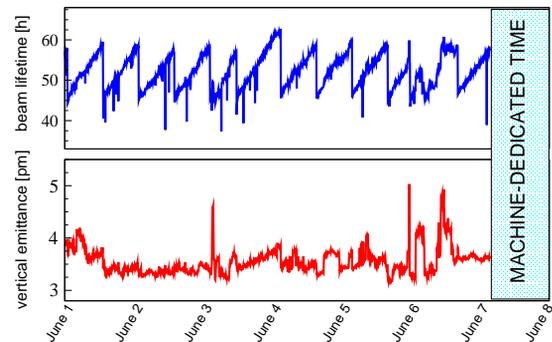
Figure 5: Beam lifetime (top) and mean vertical apparent emittance  $\bar{\epsilon}_y$  (bottom) measured during a week of beam delivery (200mA with 7/8 filling mode) in June 2011. Data acquired during refills are not displayed.
