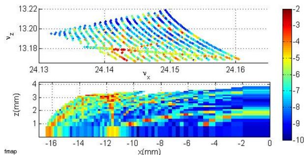
Figure 4: Frequency map analysis for the low emittance mode with multipole errors and physical limitations.
