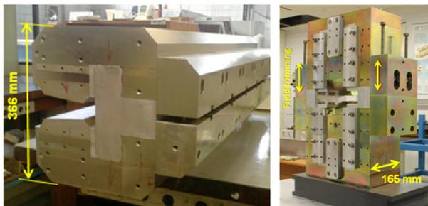
Figure 5: Prototypes of the 0.5 Tesla (left) and the 2.0 Tesla (right) permanent magnet dipoles, based on NdFeB.
