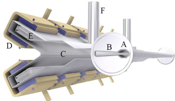
Figure 6: Proposed vacuum chamber for Sirius. A) electron beam chamber. B) Attenuation channel. C) Ante-chamber. D) Ion pump magnets. E) Ion pump cells. F) Ti sublimation pumps.
