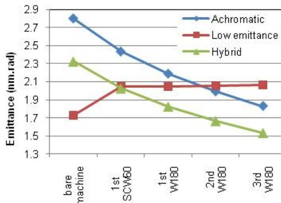
Figure 3: Effect of insertion devices on the natural emittance for Sirius three operation modes.
