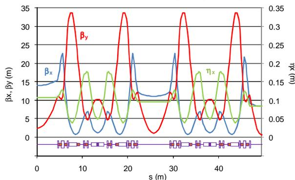
Figure 2: Optical functions of 1/10 of Sirius low emittance mode with distributed dispersion.
