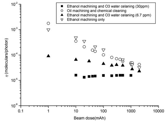
Figure 2: Photon-stimulated desorption (PSD) results with various surface treatments.
