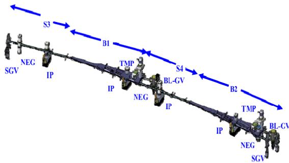
Figure 1: Assembly drawing of a vacuum system in one unit cell, excluding S1 and S2 chambers.
