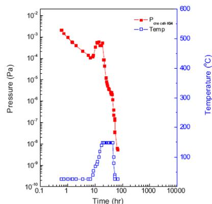
Figure 5: Pressure curve for unit cell vacuum system.
