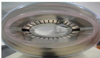
Figure 4: Bellows with RF-finger.
