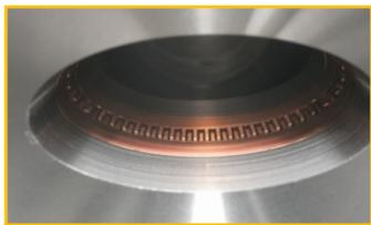
Figure 3: Sector gate valve with come type finger.
