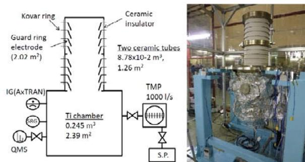
Figure 1: Schematic diagram of a presently assembled 500 kV DC gun vacuum system and its photograph.
