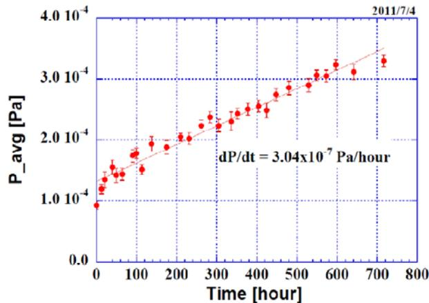
Figure 2: Raw data of the RoR measurement for assembled dc gun system by the SRG for about 1 month. The value of pressure is equivalent for nitrogen.
