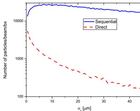
Figure 2: Bunch length dependence of the yield of the coherent pair production mechanisms.
