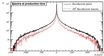
Figure 3: The spectrum of incoherent muons and electron-positron pairs. Note that the muon production cross section has been scaled up by a factor  $10^4$  to bring the processes to the same scale. These are the spectra of leptons before any tracking in the beam-beam field.
