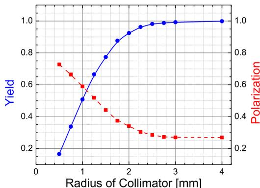
Figure 6: Positron polarization and yield normalized on yield in case of no collimator has been used versus collimator radii.
