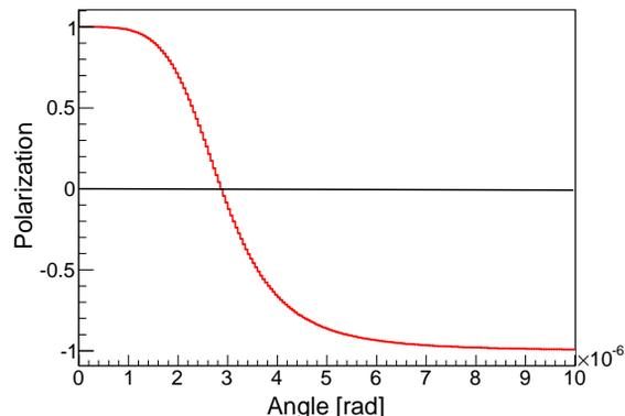
Figure 4: Photon polarization (mean value of z-component) versus angle for undulator with  $K = 0.92$  and  $\lambda = 11.5$  mm placed at 250 GeV.
