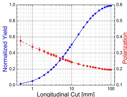
Figure 3: Positron yield and polarization versus longitudinal bunch length cut. Yield has been normalized on its value without cut.
