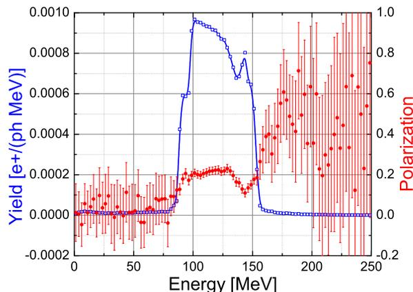
Figure 2: Positron yield and polarization versus positron energy after the capture RF (approx. 10 m long).
