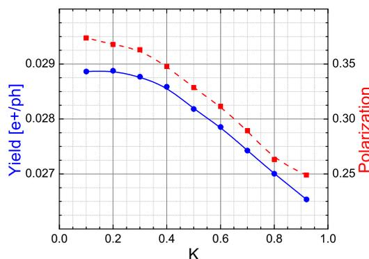
Figure 9: Positron yield and polarization vs undulator  $K$ -value.
