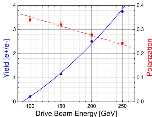
Figure 1: Yield and polarization versus drive beam energy for source with QWT (max 1 T) and without photon collimator.
