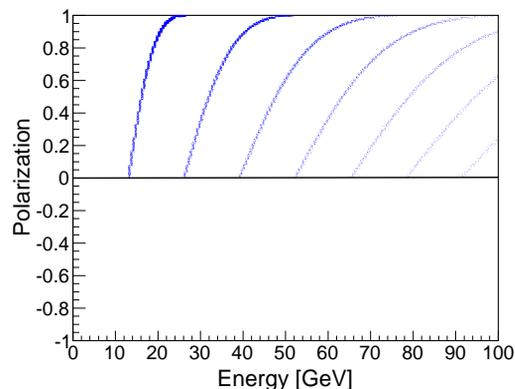
Figure 5: Polarization of photons in different harmonics (starting from 1st – left curve to 7th – right) for the angles less than  $2.8 \mu\text{rad}$ .
