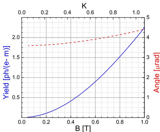
Figure 7: Average angle of photons (red dash line) and undulator photon yield per electron and one meter of undulator (blue solid line) versus  $B$ -field on axis and  $K$ -value. Undulator period is 11.5 mm.
