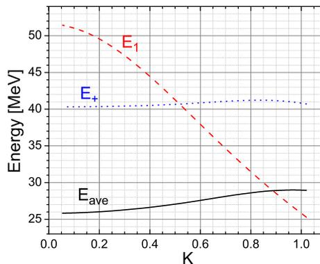
Figure 8: Average photon energy (black solid curve), energy cut-off of 1st harmonic (red dash line) and mean energy of photon with “positive helicity” only (blue dot line) vs  $K$ -value.
