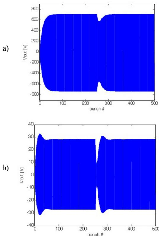
Figure 2: Phase monitor time response: a) tuned and b) detuned version.
