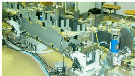
Figure 3: Supporting and pre-alignment system for two test modules type 0 in the laboratory.
