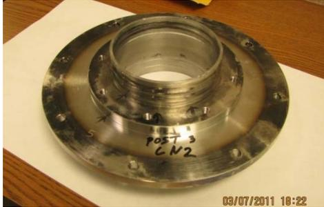
Figure 6. The world first sample of Nb-SS bimetallic transition element at the leak tests in FNAL.
