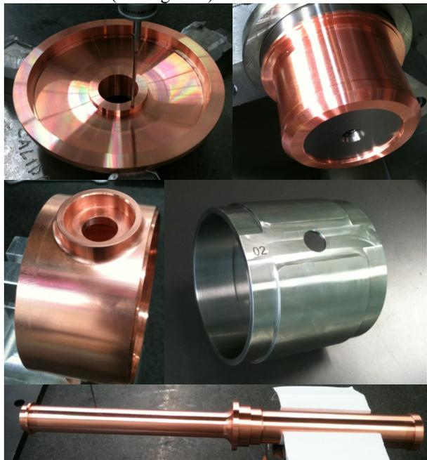
Figure 9: Different parts of the drift tubes for Linac4.
