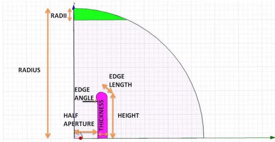
Figure 1: Geometric parameters for a cylindrical vacuum chamber and flat electrodes.
