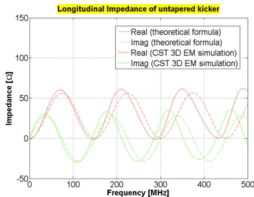
Figure 5: Longitudinal beam impedance: comparison of analytical equations for the untapered striplines with CST prediction.
