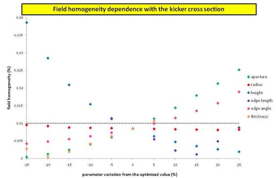
Figure 4: Field homogeneity sensitivity to the cross section parameters variation.
