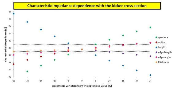
Figure 3: Characteristic impedance sensitivity to the cross section parameters variation.
