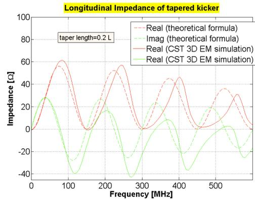
Figure 6: Longitudinal beam impedance: comparison of analytical equations for the tapered striplines with CST prediction.
