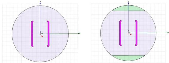
Figure 2: Flat electrodes in a cylindrical vacuum chamber (left) and in a racetrack type vacuum chamber (right).
