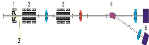
Figure 3: Schematic layout of AREAL 20 MeV S-Band linear accelerator. 1- RF –photo gun, 2- laser, 3- S-Band accel. sections, 4 –spectrometer, 5 - Beam dump.
