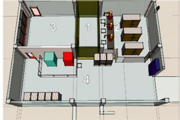
Figure 1: The AREAL supply infrastructure. 1- Laser room, 2- Klystron room, 3 –Control room, 4 - Auxiliary systems.
