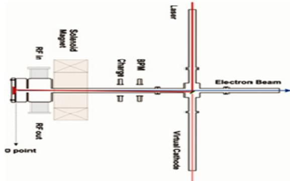
Figure 4: The layout of the photocathode RF gun section.
